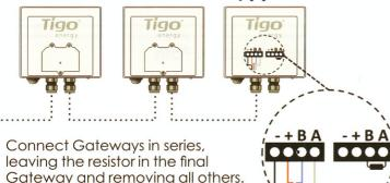
Verify wiring polarity before connecting Gateway(s) to CCA. Connect Gateway wires before powering on CCA.
