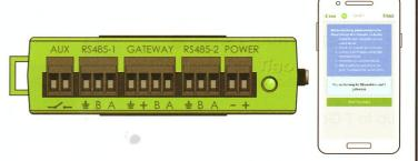
Use the Tigo SMART app to configure the Internet connection (wired Ethernet or Wi-Fi.) Select **Start Discovery** in the app to begin scanning for smart modules or add-on devices.
