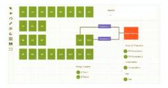
To create a map of the system that matches the physical layout, remove the peel-off stickers from the smart modules\* or record the barcodes on a map that represents their physical location.
