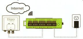
The Cloud Connect Advanced requires AC power, an Internet connection (Ethernet or Wi-Fi), and an RS-485 communication cable connection to the Gateway(s).
