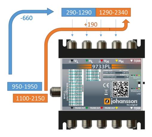
In both the Quattro and Wideband mode, the 9733PL/9734PL will allow powering the LNBs on both vertical trunks lines (see chapter 2.3 "DC Power" for more details on how to power the units and the LNB).
