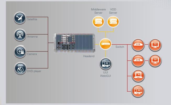
The ProStreamer system enables the distribution of DVB-S2, DVB-T and Audio-Video (Camera, DVD player, iPod,...) services over an IP-based network. Each 19" sub-rack can contain up to 9 modules, resulting in 144 programs!
